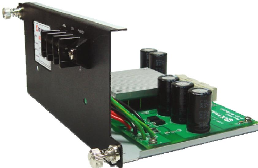
The Power Jack of XCP-DC-300 & XCP-DC-100 is 3 Terminal Connectors: -48V, OV, FGND. The Terminal Connector -48V and OV have a screw to fix an external power source cable. The FGND also has a screw, but this screw should be fixed with an external cable connected to the ground.
