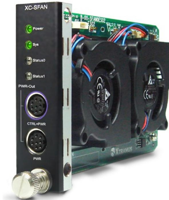
The **XC-SFAN** comes with your MCS-2160 chassis, and shall be installed on the **Fan** slot located on the far left side of MCS-2160 chassis. This module card provides ventilation for the MCS-2160 chassis.
