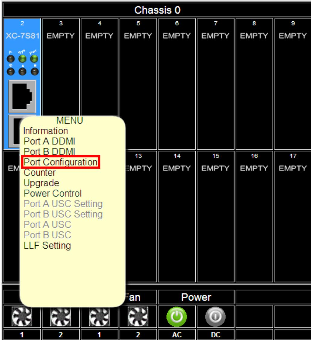
The XC-7S81 module card management doesn't include the **Port A /B USC Setting** and **Port A/B USC** function.
