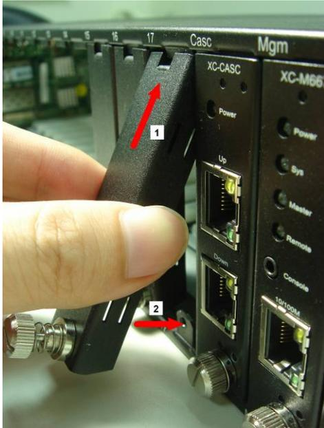
After attaching the Bracket's Latch on the internal face of Chassis' Latch, let this point be a fix central rotation point and push the bottom part of Bracket into MCS-2160.
