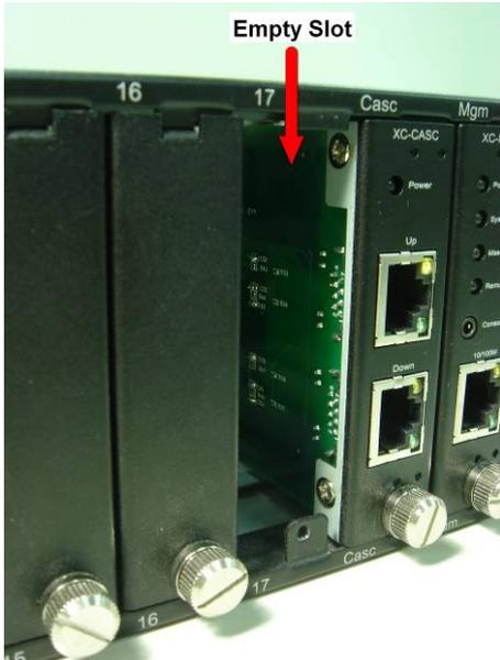
First of all, you must have an Empty Slot for the Installation of a Bracket.
